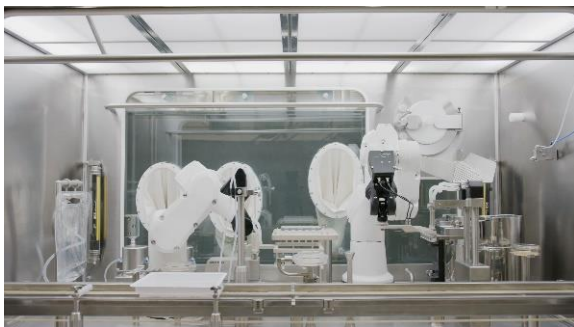
The GENiSYS R fill/close module during vial processing.
