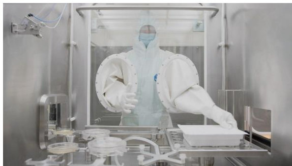
An operator manually transfers containers into a tub opening module – a task which can optionally be semi- or fully automated. Operator safety and product sterility are ensured.
