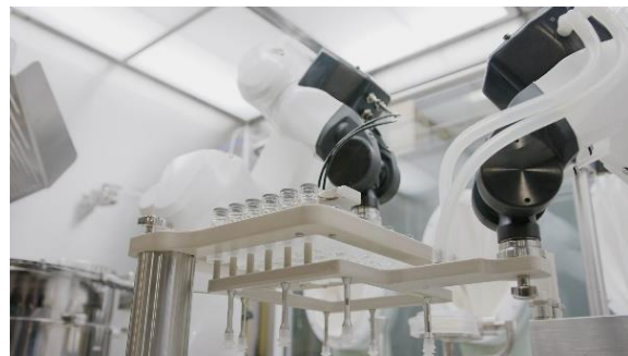
Stäubli robots hard at work filling and stoppering a nest of ready-to-use vials.
