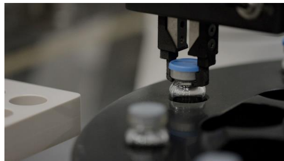
A robotic arm prepares to place a finished vial back into the nest.
