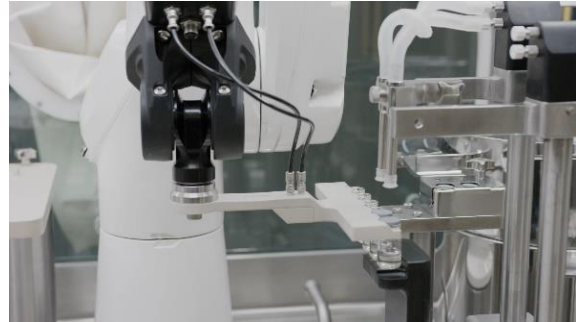
A Stäubli TX2 series Stericlean robot presents vials for secure stoppering with reliable repeatability and no risk to the aseptic environment.
