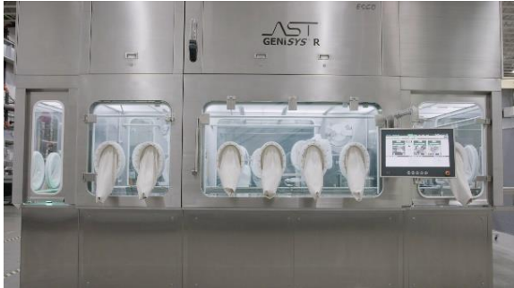
Front view of isolated GENiSYS R aseptic small batch filling and closing machine, showing glove ports and the ASTView human-machine interface (HMI).
